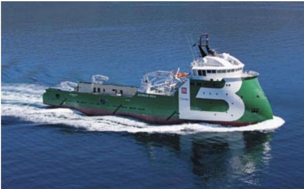
Skipsrevyen's 2006 "Ship of the Year", the Bourbon Orca , features Ulstein's X-Bow design and has won top honours for stability, fluidity and environmental performance.
