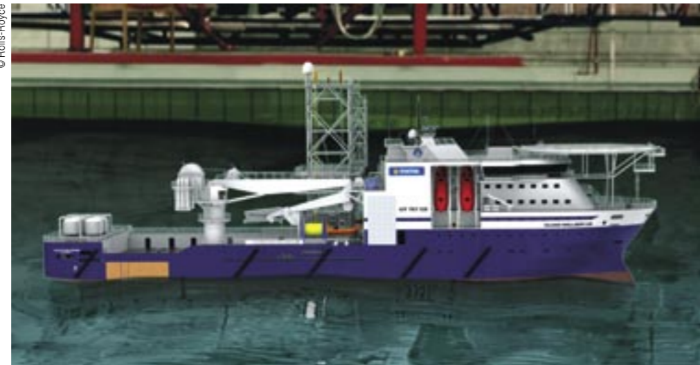
A model of the UT 767 CD oil well intervention vessel at the MARINTEK test facilities in Trondheim. The ship's design makes it possible to extract more oil and gas from wells in a cheaper, safer and simpler way.
