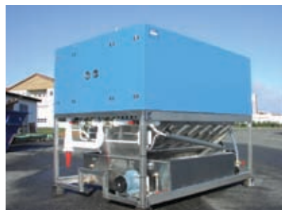
Finsam Plate Ice Machine, capacity 30 tonnes per day.
