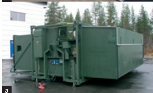
2. Expandable ISO 10' shelter for Link 16, expanded.
